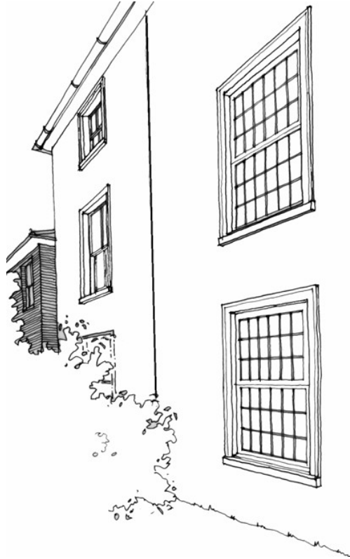
Fig. 17 Replacement windows (right) contrast sharply with the originals (left) not only in the number of panes but also in their detail. The 'glazing bars' in the double-glazed windows (right) are made of strips of plastic inserted between two sheets of glass and bear no relation to real glazing bars, and the window seems flat and lifeless. It is as if the manufacturers never learned to use their eyes.
