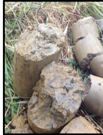
WS1 – possible shear plane at 0.85m
